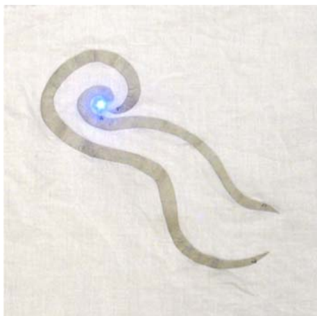
Fig. 5 A hand-cut iron-on circuit. The LED and power supply were stitched to the traces with stainless steel thread
