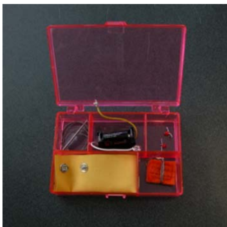
Fig. 15 A first attempt at a simple do-it-yourself e-textile kit consisting of a needle threaded with conductive thread, a snap-on battery, a fabric switch and stitchable LEDs
