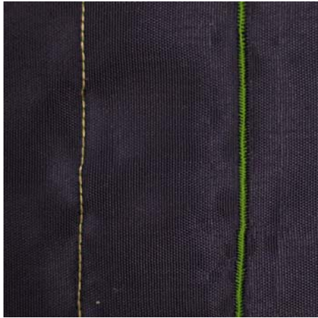
Fig. 12 An exposed trace sewn in stainless steel thread, and a similar trace covered with a couching stitch
